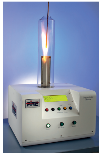
Limited-Oxygen-Index-Messung am Fraunhofer ICT
